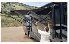
**Adjustable pitch** Choose from six settings for maximum shade and rain release. The Eclipse has the highest head clearance of any vertical arm awning.
