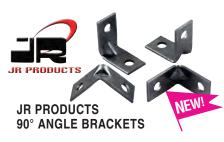
Small enough for easy concealment and the center gusset adds extra strength and stability. Constructed of high-quality steel and won't break or be affected by temperature changes. Great replacement for plastic brackets found in many RV and marine applications. Includes four brackets and eight #6 x 1/2" Pan head screws.
