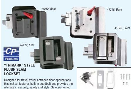
Designed for travel trailer entrance door applications, this lockset features built-in deadbolt and provides the ultimate in security, safety and style. Safety-oriented design provides exit from inside should unit accidentally be locked. Set includes 2 brass keys and all mounting screws. Cut-out size 3-3/4" H x 2-3/4" W. Installed, visible trim edge is 4-3/8" H x 3-1/2" W. Accommodates door thickness from 1-1/4" to 1-1/2".
