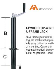
Atwood Top-Wind A-Frame Jack: **70496** 2000 lbs. Capacity; A=2.0" Retracted, 17.1" Extended; B=13.2"; C=7.0" (can use **70088** Caster, or **70082** Foot if extension tube is  $6^3/_4$ ") #80401 1
