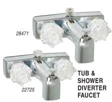
Tub and shower diverter, 4" centers with built-in anti-siphon mechanism and outlet for hand-held
