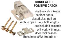
accept standard cabinet knob. (Knob not included.) Reversible strike works with flush or inset doors. Works on drawers too. Zinc. Mounting screws included.
