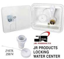
Will accommodate gravity or city water hookups. City fill has a 1-piece check valve 1/2" MPT. Easy installation, low profile and will fit in any wall. 6.5" x 7-5/8" outside dimensions;  $4\frac{3}{4}$ " H x  $5\frac{7}{8}$ " W cut-out dimensions.
