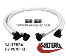
These flexible high-pressure pigtails absorb the initial surge of pressure when your pump cycles on and off eliminating noises like water hammer associated with your rigid fresh water plumbing. Includes two high-pressure hoses 1/2" x 36" and two nylon fittings for adapting female threaded fittings.
