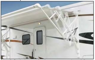
Automatically retracts your awning when canopy movement exceeds the predetermined threshold, protecting your awning when you're not around.
