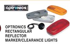
Rectangular clearance or side marker light with a reflectorized lens, eliminating the need for a separate reflector to meet DOT requirements. Twist-in socket contains both lead wire and ground wire for mounting to all surfaces. Features snap-on, replaceable lens and easy to change replaceable bulb. All-weather molded plastic housing and durable lens protect against corrosion. Dim.: 2" x 4" x 1-1/8" deep.
