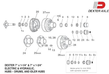
Brake, Axle Parts & Hubs
