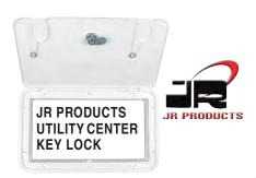
Large electrical hatch comes with two vermin doors that accept up to a 50 Amp cord. Built with a high quality plastic that won't fade of discolour. Resists road salts and acids. Paintable to match any exterior. Cutout dim.: 6" x11-1/16"; outside dim.: 7-3/4" x 12-5/8". Polar White.
