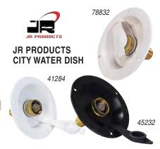
This original manufacturer's city water fill will replace any dish type water fill with a 3-1/2" opening. Brass check valve has a 1/2" M.P.T. fitting. Dish is constructed of durable plastic for a long life. Comes with a replacement rubber dust cover to keep dirt and debris from your fresh water supply. Packaged. Cut out dim. 3-1/2"; Outside dim. 4-1/2".
