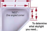
Measure the size of the rough hole opening in your roof. Skylights sit directly on your RV roof.
