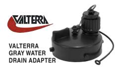
Allows for gray water sewer hook-up using 1/2" & 5/8" waste water hose. Use in conjunction with bayonet sewer fittings. Includes 3/4" garden hose connection with cap and easy thumb grip.
