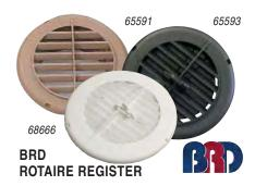
Rotaire register is molded from durable ABS plastic in a variety of colors. The damper mechanism can be easily opened and closed and may be completely removed for full flow. Grill rotates a full 360° to direct air flow where desired. 4" dia. mounting collar; overall 5" dia. by 2-1/4" D.
